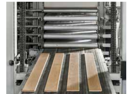
Pressing of the three tension-free solid wood layers.
