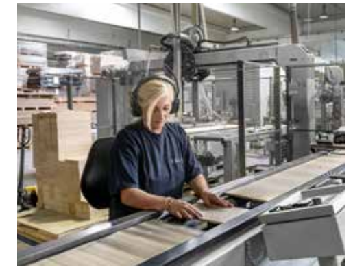
Production of the core layer from mountain spruce with quarter-sawn annual rings.
