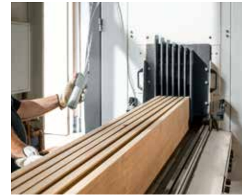
Sawing of top- and bottom layers in tension-free dry cut.
