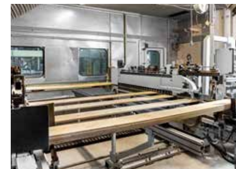
Shaping of tongue and groove for a tension-free connection of the wooden elements.
