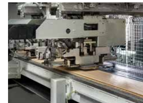
Filling of knots and cracks (especially with rustic grades).
