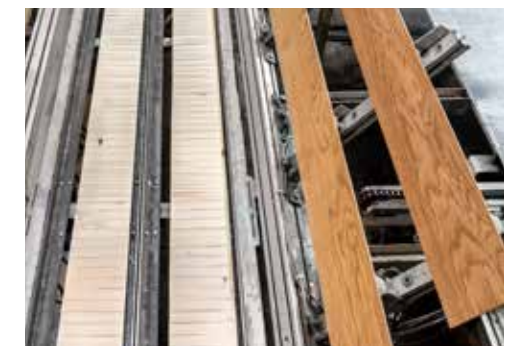
Connecting of top-, core- and bottom layer of the natural wood floors.
